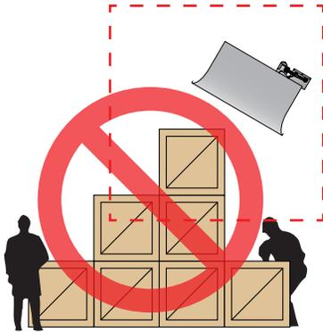
Failure to observe stated clearances to combustibles will result in a fire hazard. Failure to properly denote hazard may also result in a future hazard.
