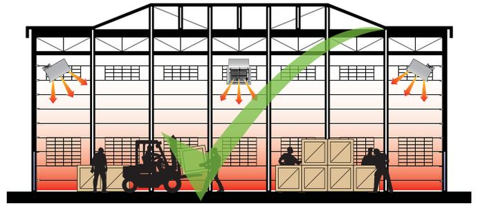
High intensity heaters are certified for commercial or industrial applications with adequate ventilation only.
