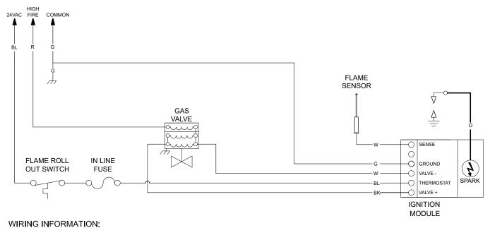
Figure 2.8 • Field Wiring Diagram
