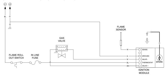
Figure 2.7 • Internal Wiring Diagram - Two Stage
