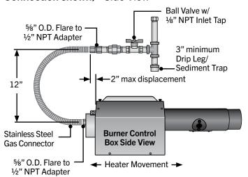
Figure 3.28 • Gas Connection (Flexible Gas Connection shown) - End View
