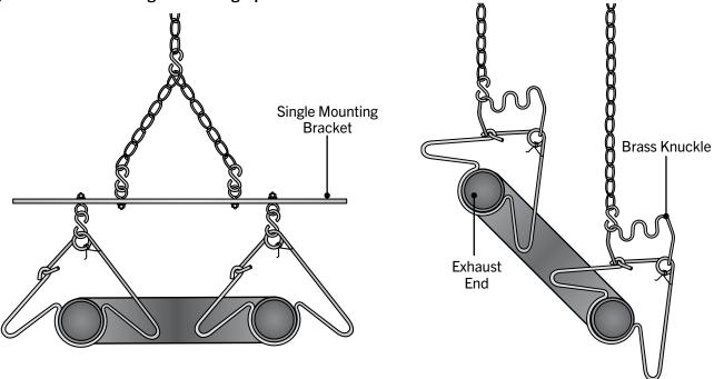
U-Tubes can be mounted from a single suspension point using an optional Single Mounting Bracket (P/N: SMB) with five S-hooks and #1 double-loop chains.
