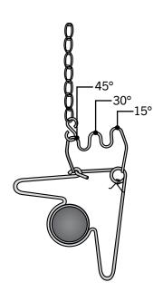
For variety of hanging angles, use an optional Brass Knuckle (P/N: BK) fitting with a #1 double-loop chain and S-hook.
