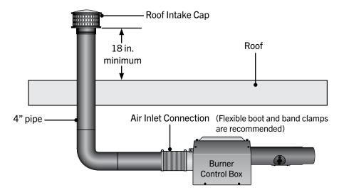
Figure 3.26 • Outside Combustion Air Sidewall Intake - Side View
