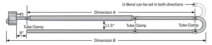
Figure 3.11 • U-Bend and Elbow Dimensions
