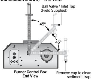
Refer to Chart 3.8 for natural gas and Chart 3.9 for propane gas to determine the cubic feet per hour (CFH) required for the type of gas and size of unit to be installed. To determine the proper pipe diameter, use the CFH value and the length of pipe necessary from Chart 3.9. In the case where several units are serviced by the same main gas line, the total capacity (CFH) and length of main must be adequate to service all appliances downstream of this main.
