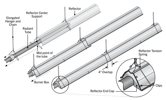
Figure 3.15 • Width of Installed Reflector - Top View
