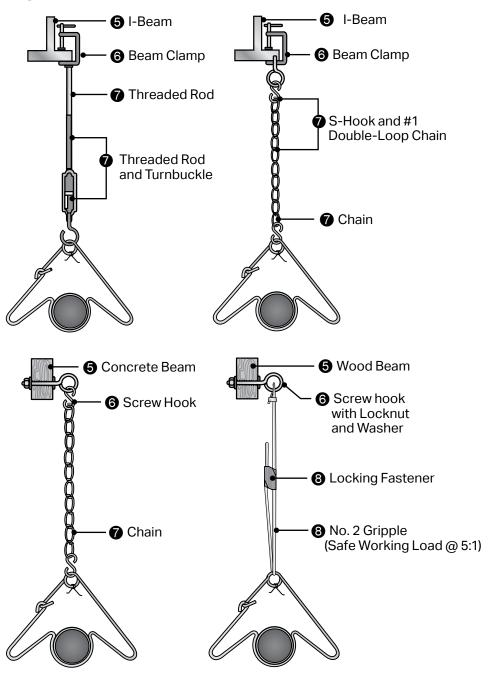
Figure 3.4 • U-Tube Hanger Mounting Options
