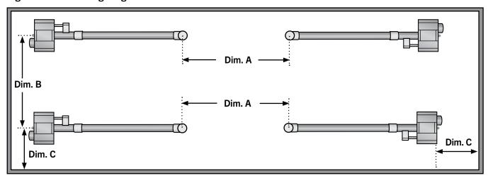
Note: Dimensions A, B, & C are based upon heaters hung at the factory recommended mounting height.
