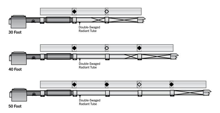
**IMPORTANT:** When securing joints on reflectors which are rotated on an angle from horizontal, secure joint only on top side of reflector to allow for sufficient heater expansion and contraction.
