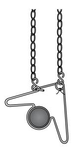
For 45° hanging angle, use two S-hooks and two #1 double-loop chains.
