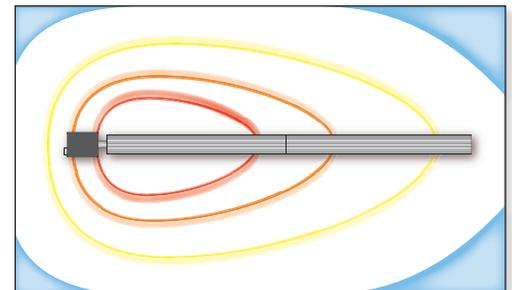
A modulating heater operating at reduced output results in a diminished comfort zone because of a shortened flame and uneven heat pattern.
