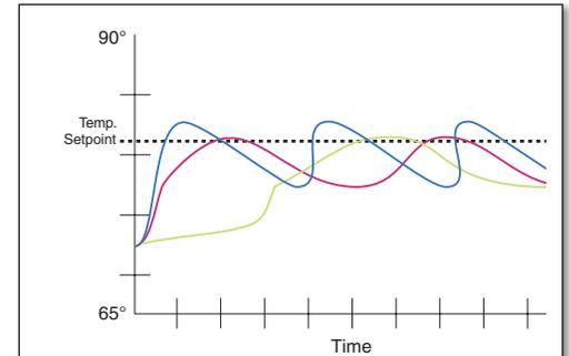
Here we see the response time of a two-stage, single-stage, and modulating heater starting from the same initial conditions.
