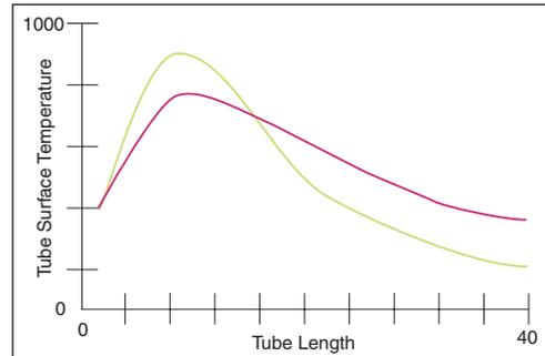
This graph depicts the temperature differential of the radiant tube exchangers over the length of the heater while operating at reduced output.
