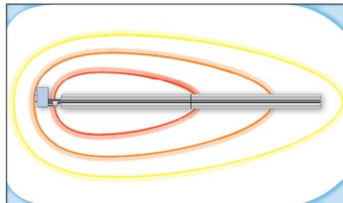
A two-stage heater operating at low fire has a greater coverage and comfort area when compared to a modulating heater because of a longer flame.
