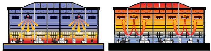
**Infrared two-stage heating system**
