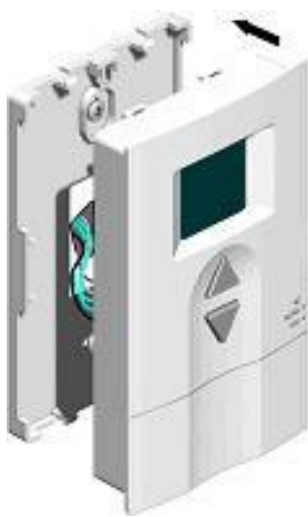
Fig.8 Installing the thermostat
