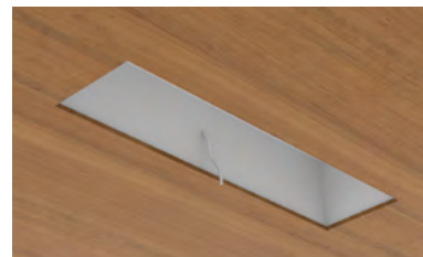
Figure 4 • Ceiling Pocket in Finished Ceiling
