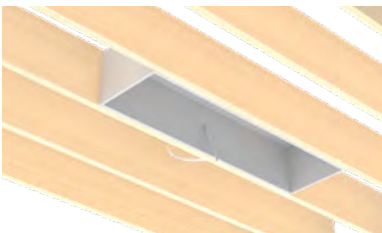
Figure 3 • Ceiling Pocket Between Framing
